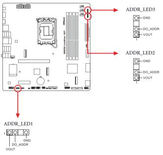
Connect your Addressable RGB LED strips to the Addressable LED Headers (ADDR\_LED1 / ADDR\_LED2 / ADDR\_LED3) on the motherboard.
