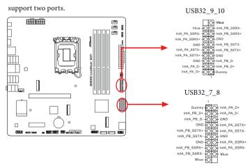
Front Panel Type C USB 3.2 Gen1 Header (20-pin F\_USB32\_TC1) (see p.6, No. 12)
