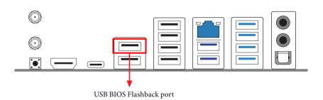
ASRock BIOS Flashback feature allows you to update BIOS without powering on the system, even without CPU.
