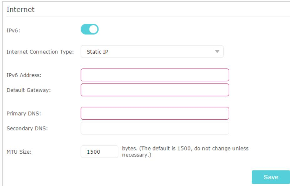
The screenshot shows the 'Internet' configuration page. At the top, the title 'Internet' is displayed. Below it, the 'IPv6' toggle is turned on. The 'Internet Connection Type' is set to 'Static IP'. There are four empty input fields for 'IPv6 Address', 'Default Gateway', 'Primary DNS', and 'Secondary DNS'. The 'MTU Size' is set to '1500' bytes, with a note: '(The default is 1500, do not change unless necessary.)'. A 'Save' button is located at the bottom right.
