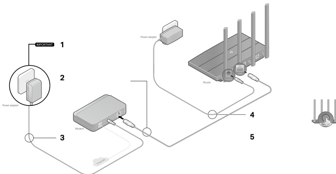
1. Unplug the modem, and remove the backup battery if it has one.
