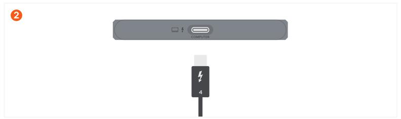
Connect the Docking Station to your host device using the included Thunderbolt 4 cable. Host port is located on the right side of the Docking Station.
