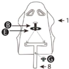
**6. Insert the backrest mount into the hole in the butterfly mechanism and secure it by turning the handle.**
