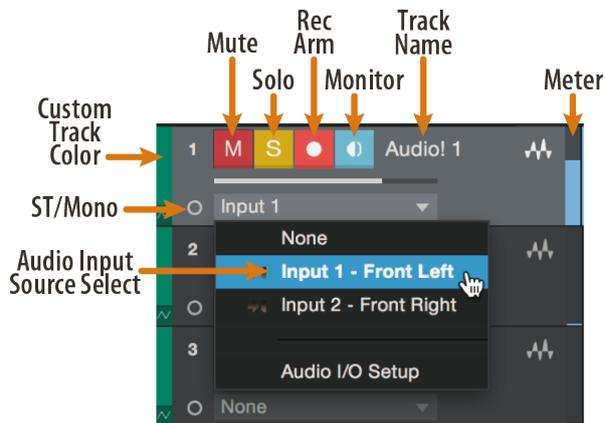
Note: Instrument tracks are nearly identical to audio tracks. The Input Source list for Instrument tracks lists available external MIDI devices as well as any virtual instruments that have been added to the Song.
