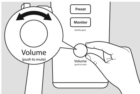
Turn the Volume knob for your Revelator clockwise while speaking into the microphone. Watching for the signal/clip indicator to turn red, then back it down until the indicator is green only. When you've stopped speaking the knob will go dark.
