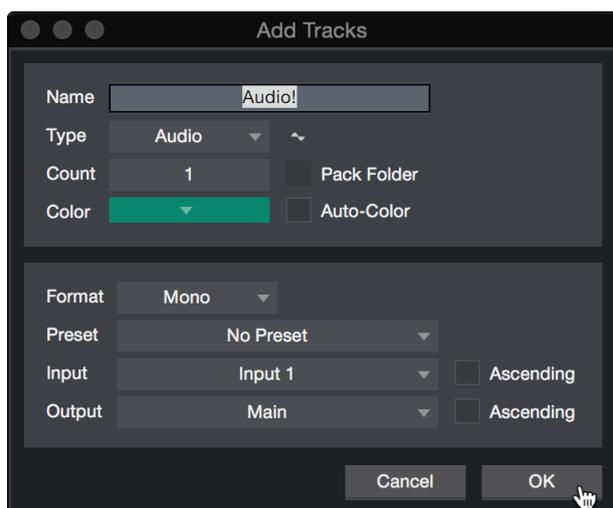
To begin recording, create an audio track from the Add Tracks window, set its input to Input 1 on your Revelator, and connect a microphone to the same input.
