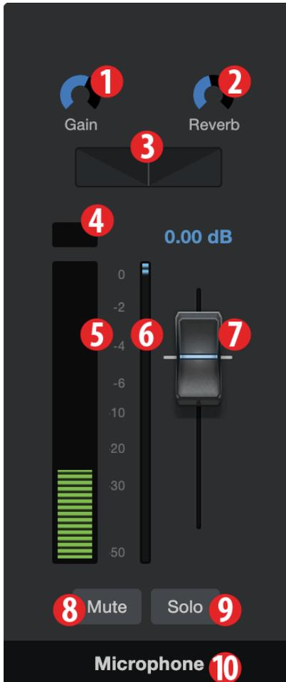
1. **Gain.** Use this control to set the gain for your connected microphone or instrument. Gain can also be set using the Encoder knob on your Revelator.
