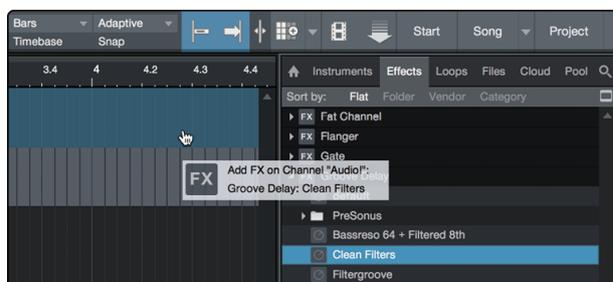
To add a plug-in effect to a track, click the Effects button in the browser and select the plug-in or one of its presets in the effects browser. Drag-and-drop the selection over the track to which you would like to add the effect.
