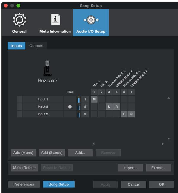
From the Inputs tab, you can enable the inputs for your Revelator, including the Loopback Inputs that you'd like to have available. We recommend you create a mono input using Input 1 of your Revelator and two Stereo Inputs; one for Stream Mix A L/R and another for Stream Mix B L/R.
