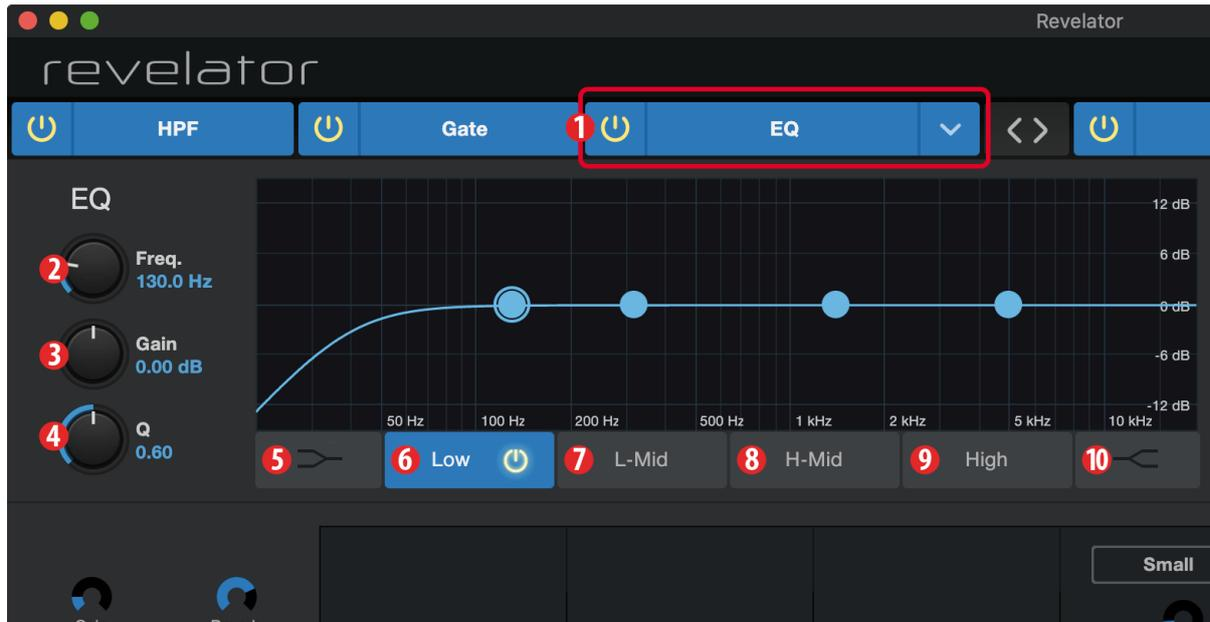
1. **On/Off.** Turns the EQ on or off in the signal chain.
