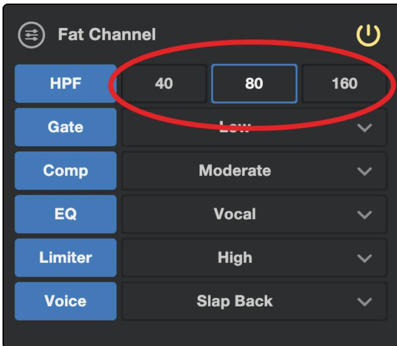
**Power User Tip:** When looking at frequency ranges in audio, it's important to know that the smaller the number, the lower the frequency is. The 40 Hz and 80 Hz settings can be especially useful in reducing the “rumble” from a nearby road or any background electrical noise or hum.
