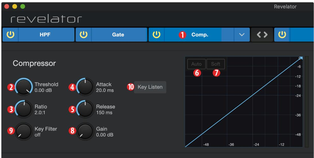
1. **On/Off.** Turns the Compressor on or off in the signal chain.
