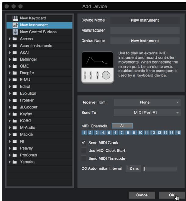
Select your device in the menu on the left. If your device is not listed, select New Instrument. At this point you can customize the name of your keyboard by entering the manufacturer and device names.
