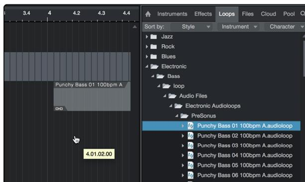
Audio and MIDI files can be quickly located, auditioned, and imported into your Song by dragging them from the file browser into the Arrange view. If you drag the file to an empty space, a new track will be created with that file placed at the position to which you dragged it. If you drag the file to an existing track, the file will be placed as a new part of the track.
