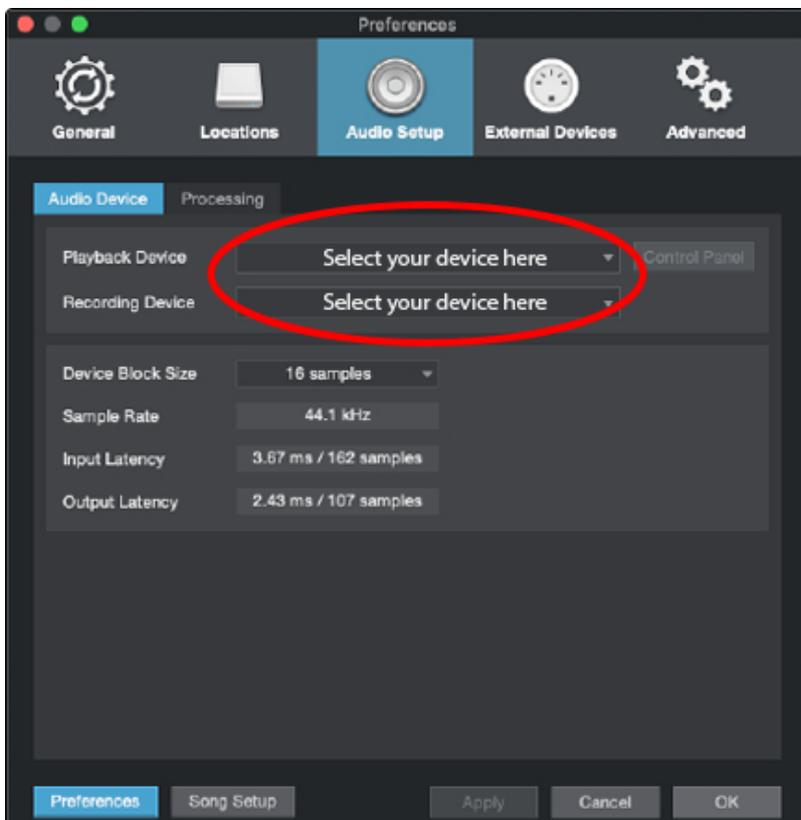
In the Options window, click on the Audio Setup tab and select your device driver from the pull-down.
