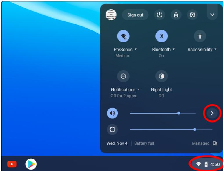
2. Select the greater than symbol (>) to the right of the volume slider to enter Audio Settings and select your audio device. The green circle with the check mark indicates your preferred device. If Revelator is not already selected, select it here for both Output and Input.
