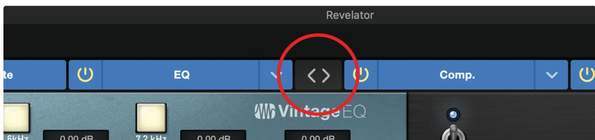
**Power User Tip:** Placing the compressor before the EQ allows you to make dramatic changes to the EQ settings without needing to alter the compressor setting. However, if you place the EQ before the compressor, you can better control different frequencies, achieving a more natural response.
