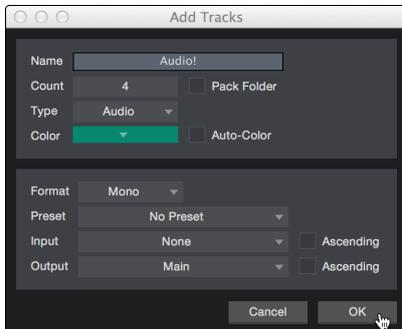
In the Add Tracks window, you can customize the track name and color, add a preset rack of effects, and set the physical source for the input and output of your audio tracks. Most important, you can select the number and type of tracks you'd like to create.
