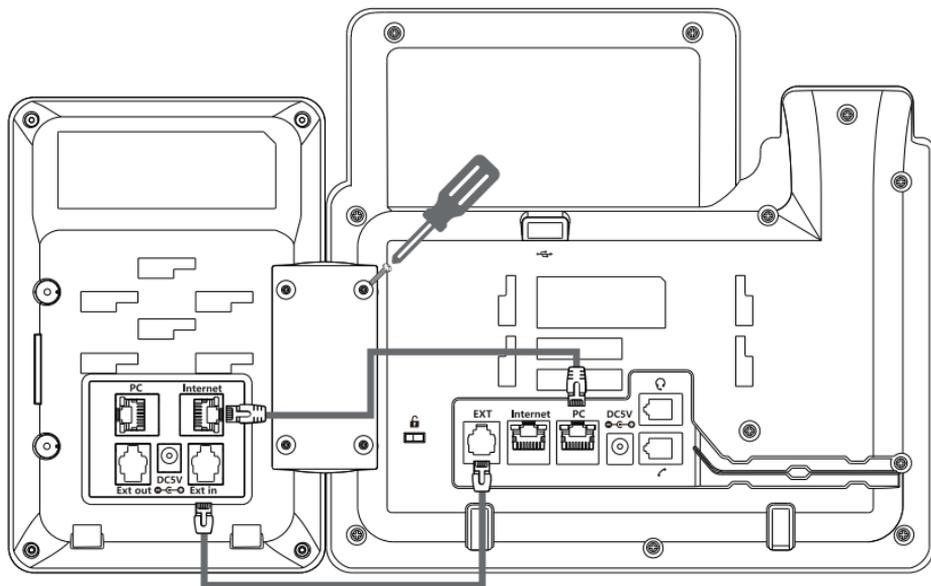
Connecting two or more expansion modules on a single IP phone is shown as below:
