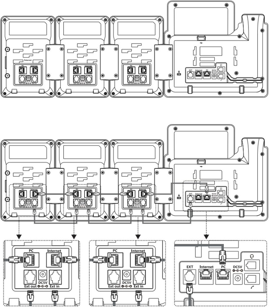
Note: The electricity of module has been automatically provided from the IP phone to the expansion module(s) upon connection. If you want to use more than one expansion modules on a single phone, you need to connect an additional power adapter (5V/1A) to any one of the expansion modules.
