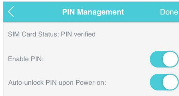
4. Once enabled, you can save the trouble of entering the PIN code on your Mobile Wi-Fi upon power-on.
