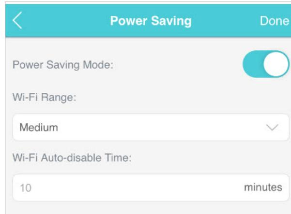
3. Tap **Done**. If there are no devices connected to the Mobile Wi-Fi for the time you specified, the Wi-Fi will be disabled automatically.
