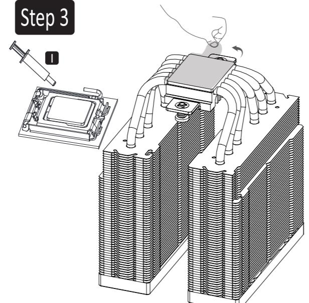
**EN** Apply thermal conductive paste to the CPU and remove the protective film from the copper substrate
