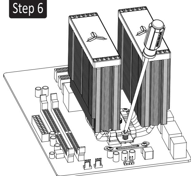
**EN** Place the heat sink on the CPU and fix it on the installation fastener
