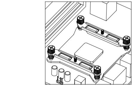
**EN** Install the 2011 screw onto the CPU bracket, install the fastener and fix it with nuts
