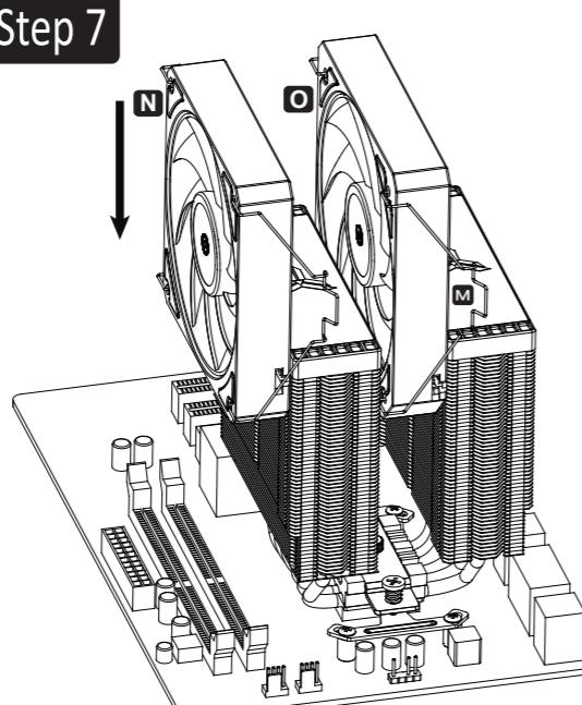
**EN** Install the fan into the module
