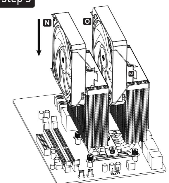
**EN** Install the fan into the module
