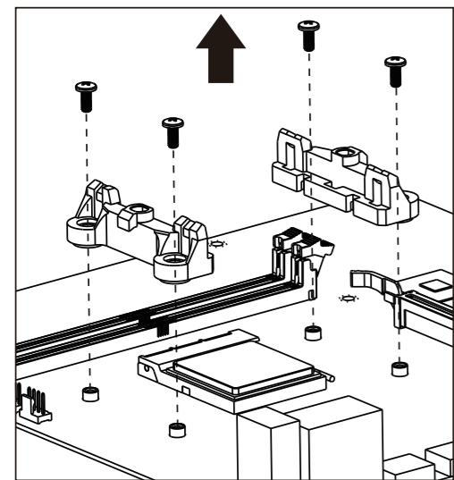
**EN** Remove the AMD mounting bracket and keep its original backplane
