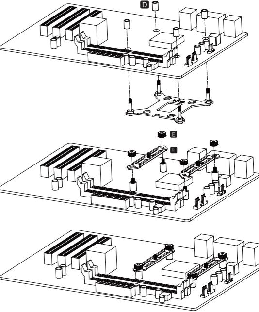
**EN** Install the back plate and fastener
