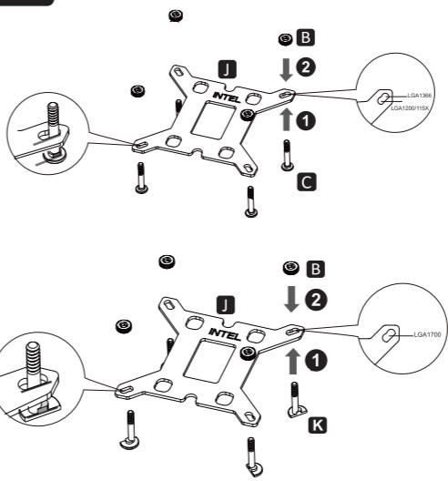
**EN** Place the set screw in the corresponding hole position of the Intel bracket, and then insert the gasket
