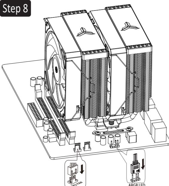
**EN** Connect the fan lead to the main board according to the figure above
