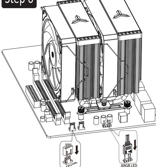
**EN** Connect the fan lead to the main board according to the figure above
