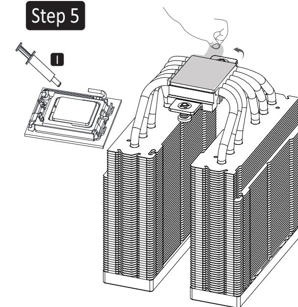
**EN** Apply thermal conductive paste to the CPU and remove the protective film from the copper substrate
