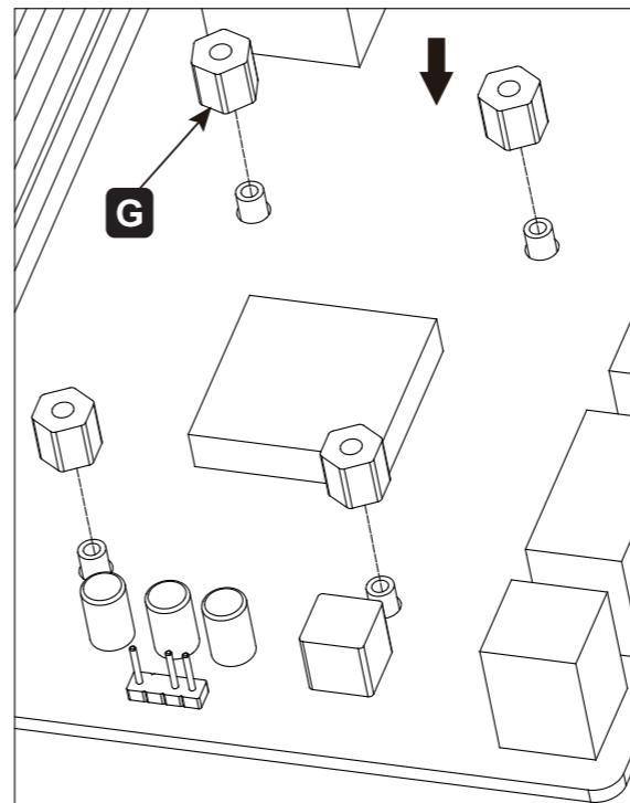
Installation of AMD spacer column
