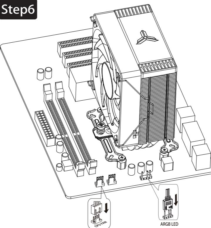
Connect the fan lead to the main board as shown in the figure above
