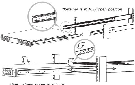
\*Press trigger down to release the slides from locking
