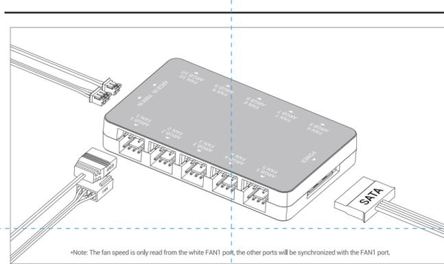
Note: The fan speed is only read from the white FAN1 port, the other ports will be synchronized with the FAN1 port.
