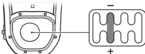
Make sure the shift lever is in the neutral position when switching to the SEQ mode.
