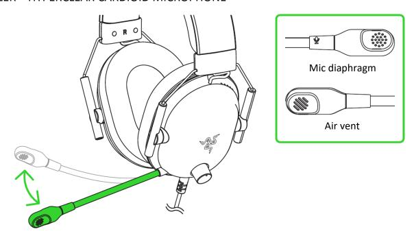
The recommended mic-to-mouth distance for optimal sound capture is 1.5 cm to 3 cm (0.59 in to 1.18 in).
