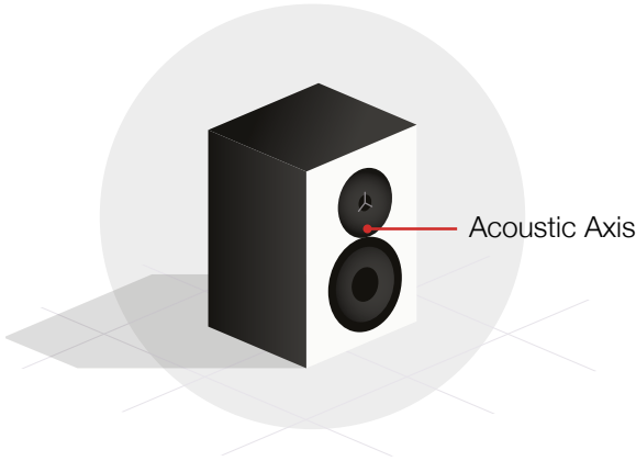
Figure 3 : The acoustic axis
