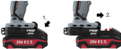
To remove the battery, press the unlocking To remove the battery, press the unlocking button and pull out the battery toward the front. **Do not exert any force.**
