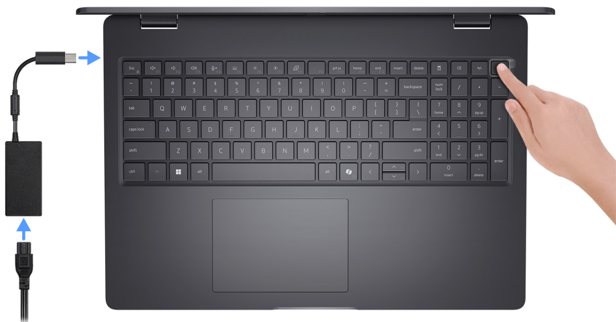
Рисунок 7. Connect the power adapter and press the power button.
