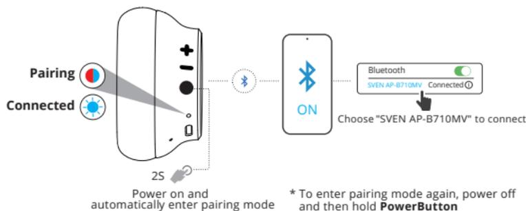
Fig. 2. Power on and connection
