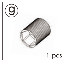
Tool for stand-off bolt
