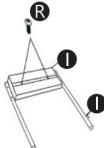
**4. Secure the footrest mount Q with the screws R over the seat G. Insert the footrest I into the mounts.**
