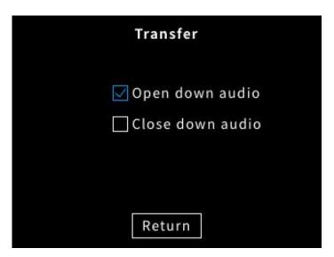
Enter the download function, you can set to turn on or off the download of the wireless unit audio, which is Not opened by default.
