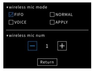
Enter the wireless microphone management mode from the conference mode on the main interface. There are 4 microphone modes, and you can switch to one of them as needed; the number of microphones is the current maximum number of microphones allowed to be opened (the range of wireless N is  $1^{8}$ ), and you can switch to one of them.
