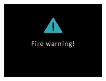
By short-circuiting the two signal pins of the ALARM output on the back of the conference host (simulating sending a fire alarm signal to the host), the conference host and unit machines enter the alarm state. When the alarm state is released, the system automatically returns to normal.
