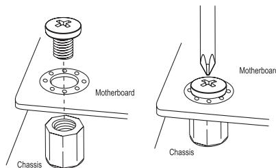
3. Locate the matching mounting holes on the chassis. Align the mounting holes on the motherboard against the mounting holes on the chassis.
