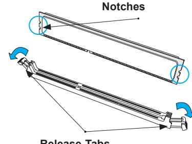
Insert the DIMM module into the memory slot.
