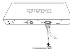
4. Circle the tie of the retainer around the power cord and into the locker of the retainer.
