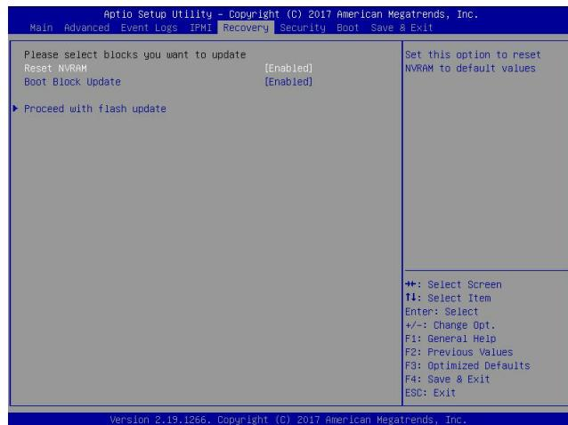
3. After locating the new BIOS binary image, the system will enter the BIOS Recovery menu as shown below:
