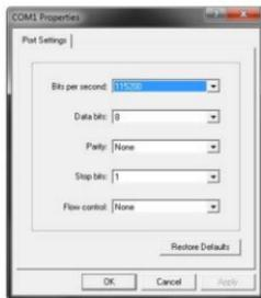
Figure 9. Hyperterminal Connection Properties
