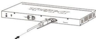
Figure 3-2. Connect the power cord to the Switch
