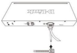
Figure 3-3. Slide the Retainer through the Tie Wrap
