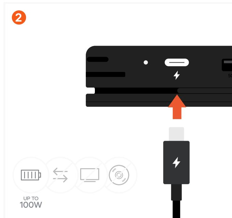
Connect USB-C charging cable to the adapter's USB-C PD charging port.
