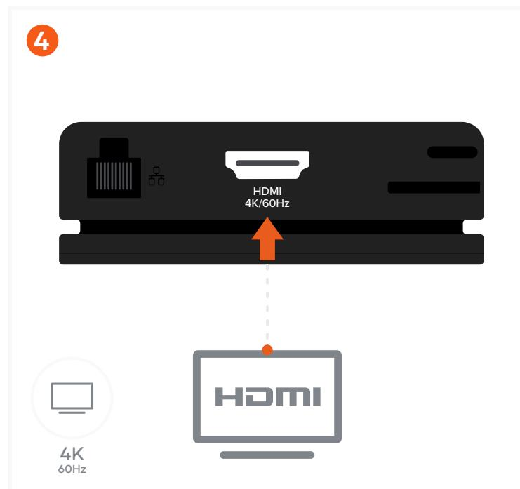
Connect HDMI cable from the adapter to a 4K HDMI-equipped display.
