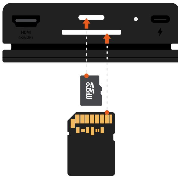
**Insert micro/SD cards into the adapter's card reader slots.**
