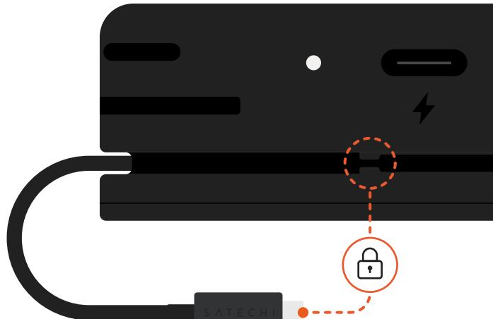
**Wrap the USB-C connector cable around the hub and secure it in place for storage.**
