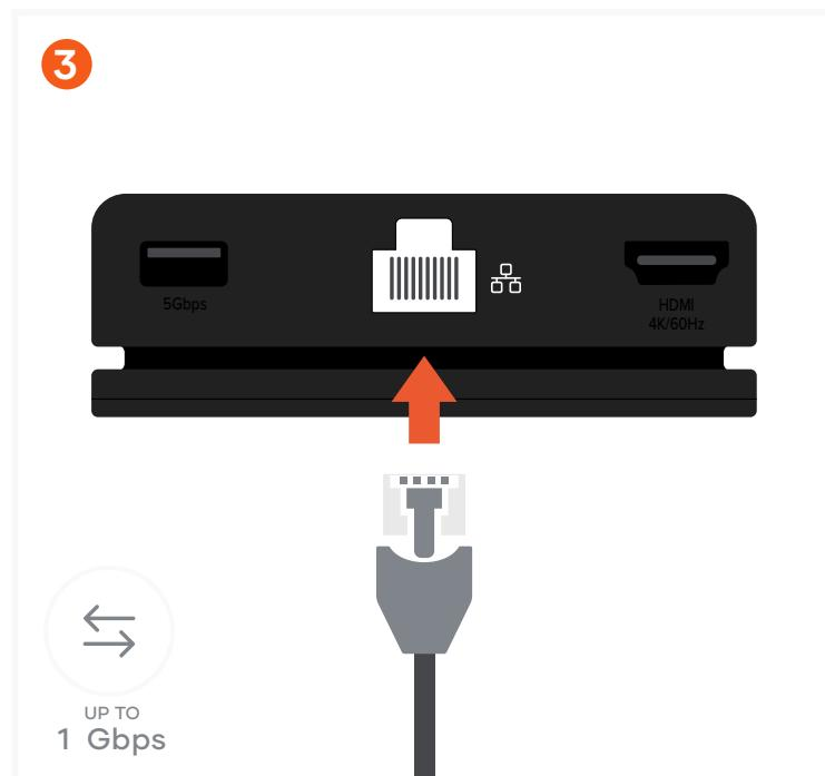
Insert RJ45 Ethernet cable to the adapter's Gigabit Ethernet port.
