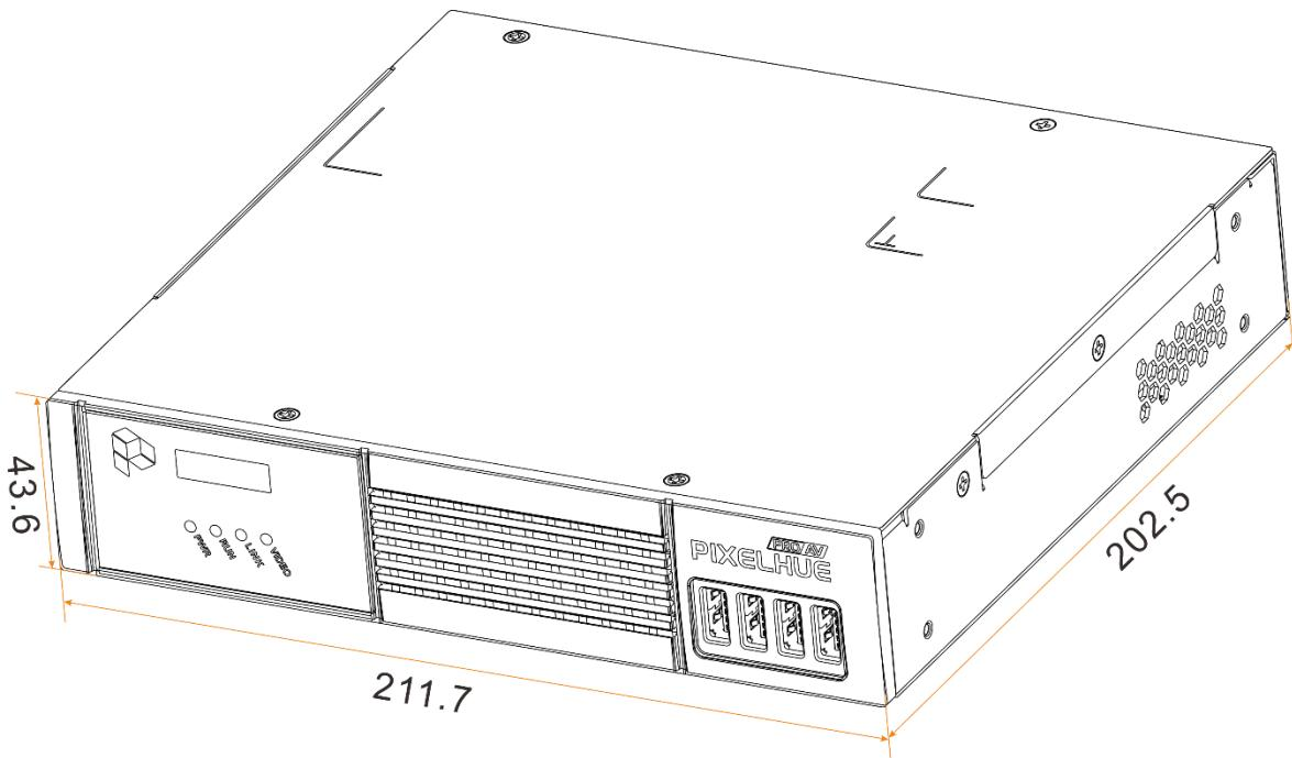
Tolerance:  $\pm 0.3$  Unit: mm
