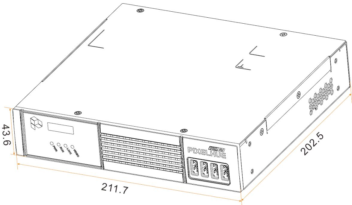
Tolerance:  $\pm 0.3$  Unit: mm
