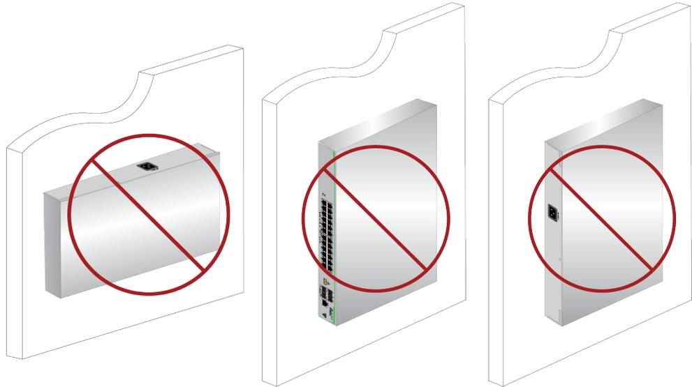
Figure 26. Incorrect Wall Installation
