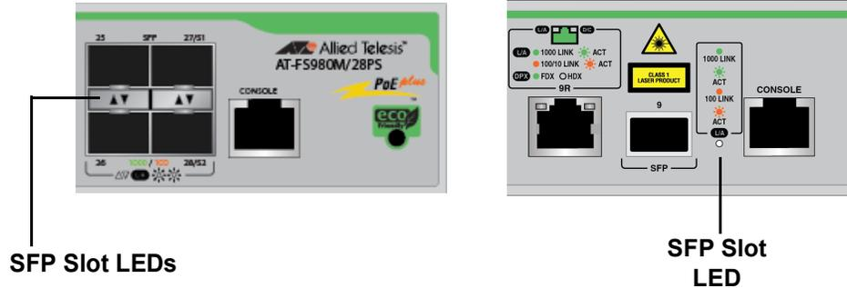
Figure 24. SFP Slot LEDs
