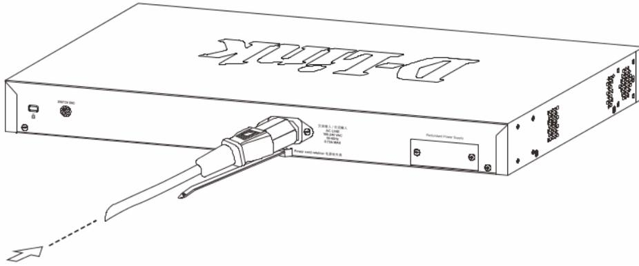
**Figure 6 — Connect the power cord to the Switch**
