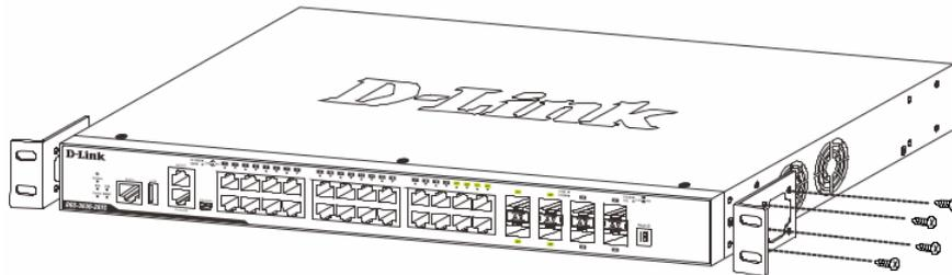
**Figure 2 — Attaching rack-mount brackets to the Switch**
