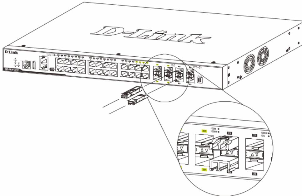
**Figure 4 — Inserting transceivers into the transceiver ports**
