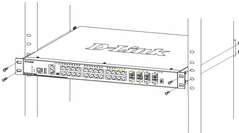
**Figure 3 — Installing the Switch in a Rack**
