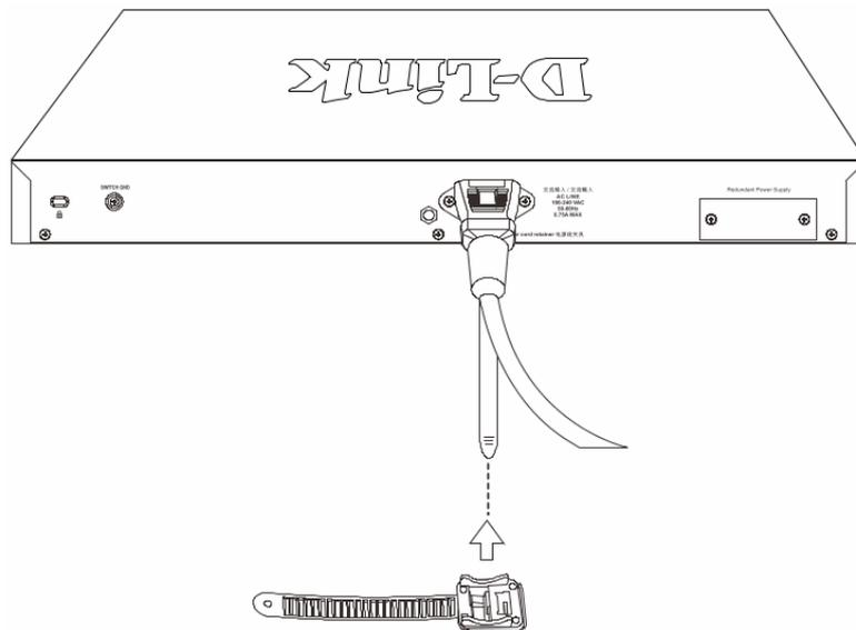
**Figure 7 — Slide the Retainer through the Tie Wrap**
