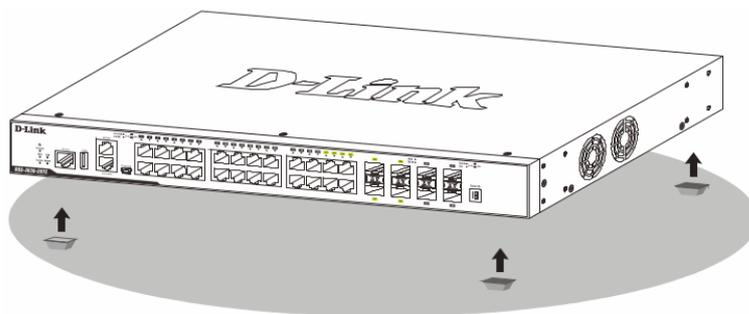
**Figure 1 — Attaching rubber feet to the Switch**
