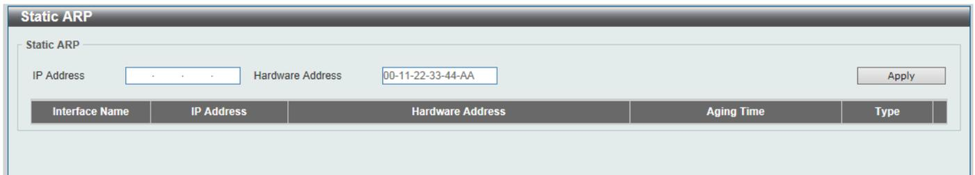
Figure 6-3 Static ARP Window
