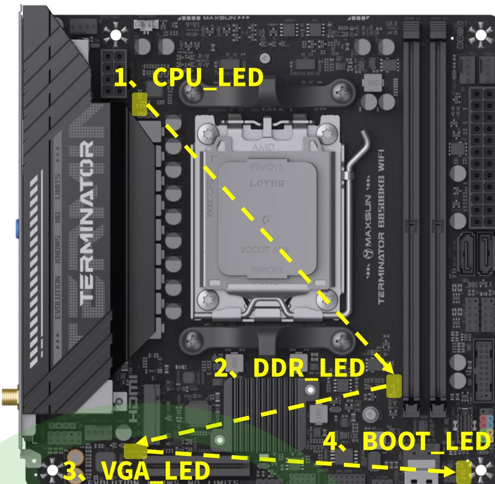
**CPU\_LED → DDR\_LED → VGA\_LED → BOOT\_LED**
