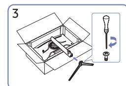
Insert the stand base into the stand neck in the direction as shown in the figure.
