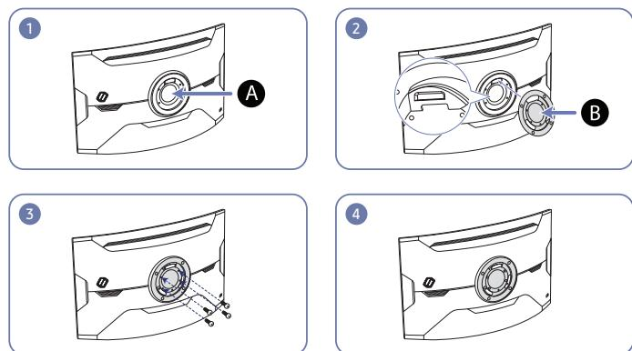
**A** Attach the BRACKET WALL here
