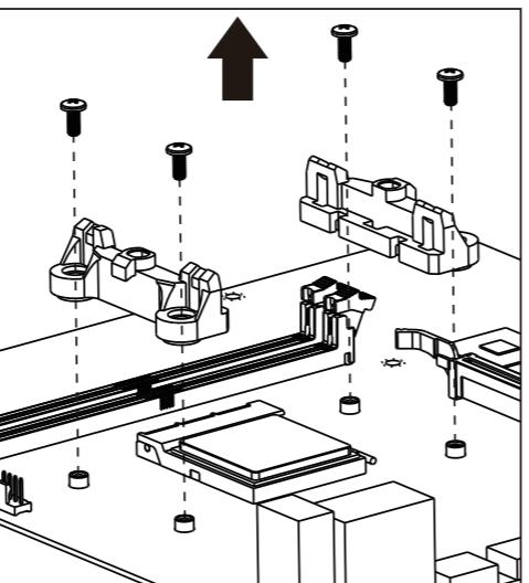
Remove the plastic retainer of the AMD retention module, place the existing backplate back to MB
