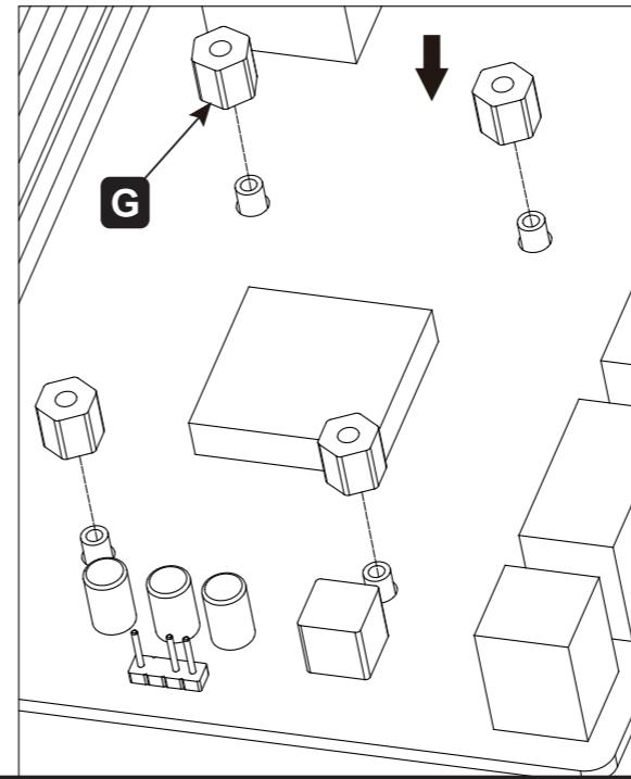
Installation of AMD spacer column
