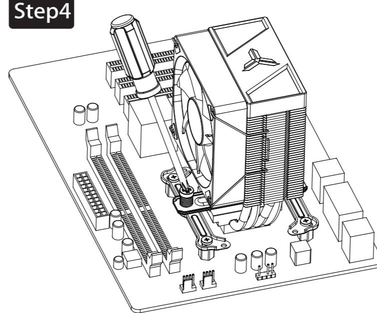
Place the cooler on the CPU while aligning the screws to the backplate mounting points, secure with screwdriver.
