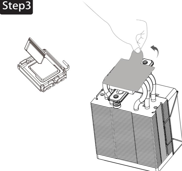
Applying the thermal paste on CPU evenly, and remove the protection film from copper base
