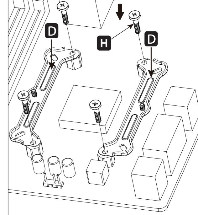
Install the mounting brackets and secure with screw
