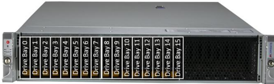
Figure 6-2. Drive Bay Configuration Options - 16 Drive Bays
