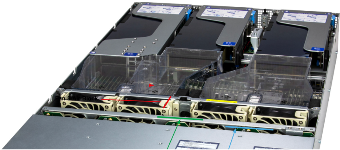
Figure 6-21. Fan 8 Air Blocks Stored; Fan 6 and Fan 4 Air Block in Blocking Position
