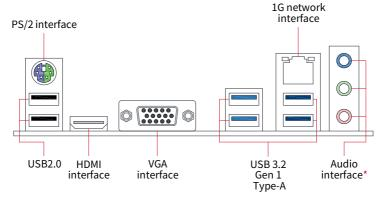
(\*Note: The blue in the audio interface is the audio input, the green is the audio output, and the pink is the microphone interface)
