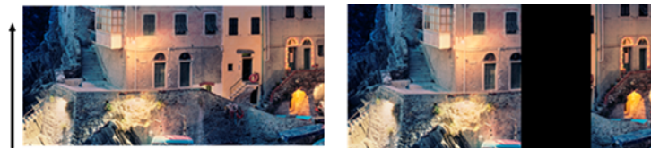
Original Scan affected by a failing scanbar
