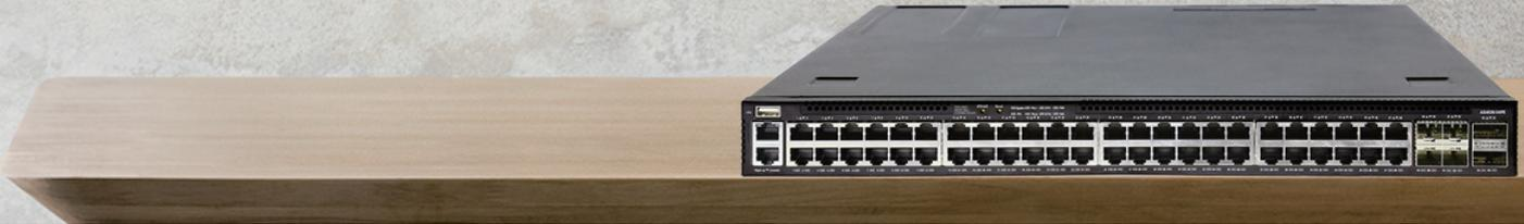
The Edgecore EPS202 is a high-performance Gigabit Ethernet L2/L3 switch featuring 54 ports; the EPS202 has 48 x 10/100/1000BASE-T ports, 4 x 10G/25G SFP28 uplink ports, and 2 x 100G QSFP28 stacking ports (stacking capability subject to NOS implementations); plus the 48 x 10/100/1000BASE-T ports fully support IEEE 802.3at and IEEE 802.3bt Power-over-Ethernet (PoE).
