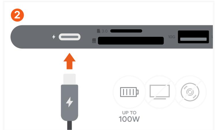
2 Connect USB-C charging cable to the adapter's USB-C PD charging port - up to 100W (15W used for operation). Does not support video output. Does not support CD/ DVD Drives or Apple SuperDrive.
