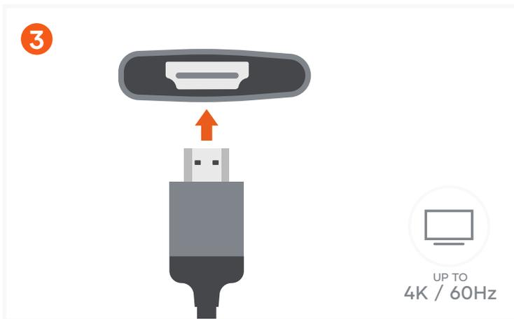
3 Connect HDMI cable from the adapter to a 4K HDMI-equipped display. Up to 4K at 60Hz. Only supports direct HDMI connections.
