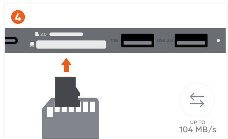
4 Insert micro/SD cards into adapter's card reader slots. Cards can be read simultaneously. Supports UHS-I read/write speeds.
