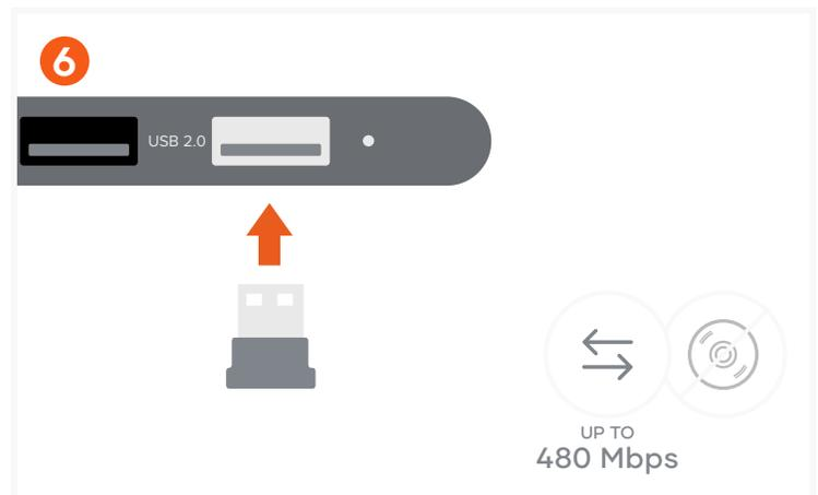
6 Connect one USB 2.0 Type-A device for low-power devices up to 480 Mbps. Recommended for USB-A peripherals or wireless receivers. Does not support CD readers including the Apple SuperDrive.
