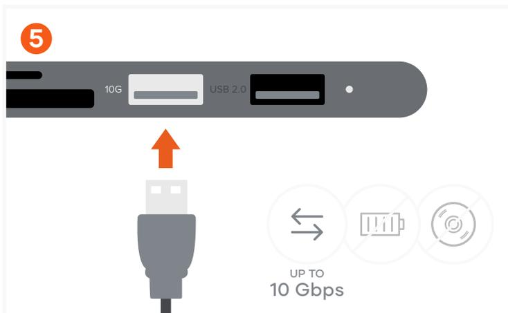
5 Connect one USB 3.0 Type-A device for high speed data transfer up to 10 Gbps. Does not support charging or CD readers including the Apple SuperDrive.
