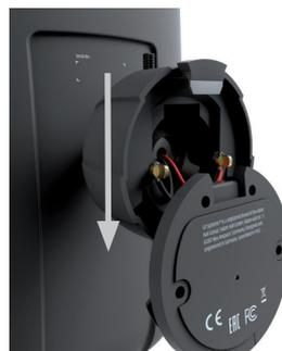
**2** Firmly secure the wall mounting plate with the terminal block at the top using suitable screws on a wall sufficiently capable of supporting the load. For speaker cables laid under plaster, the corresponding cable must be inserted through the central cable bushing prior to securing the wall mounting plate. Now connect the speaker cables to the corresponding contacts of the terminal block.
