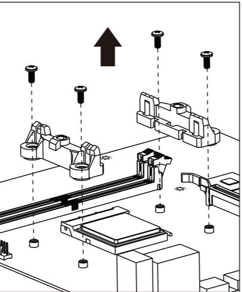
Remove the plastic retainer of the AMD retention module, place the existing backplate back to MB
