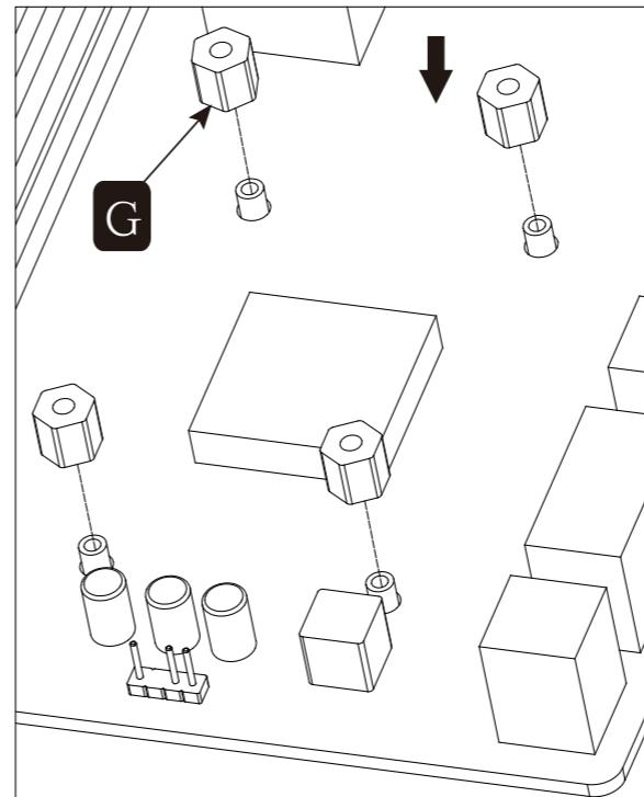
Installation of AMD spacer column
