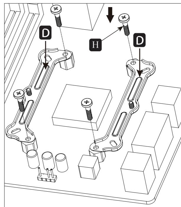
Install the mounting brackets and secure with screw
