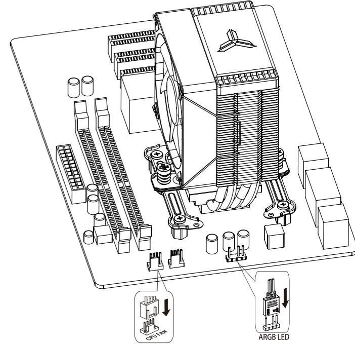
Connect the fan lead to the main board as shown in the figure above
