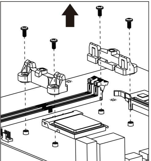
Remove the plastic retainer of the AMD retention module, place the existing backplate back to MB
