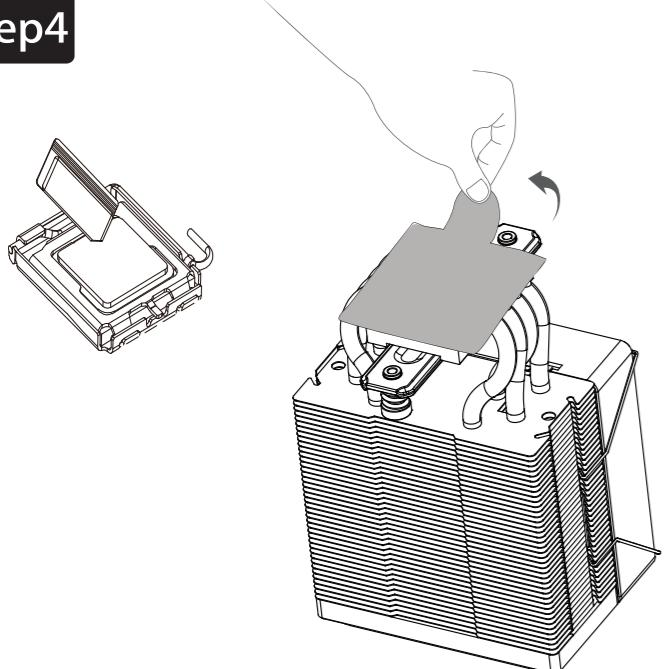
Applying the thermal paste on CPU evenly, and remove the protection film from copper base
