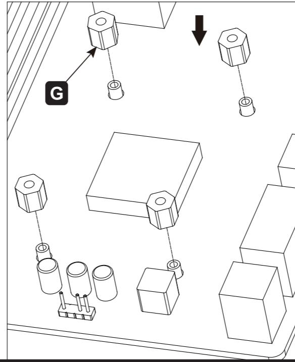
Installation of AMD spacer column
