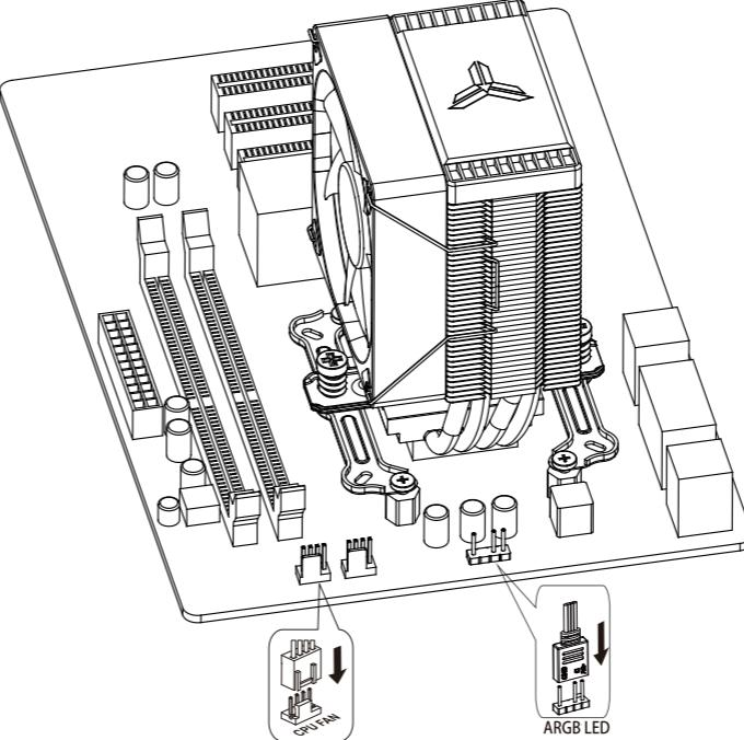
Connect the fan lead to the main board as shown in the figure above
