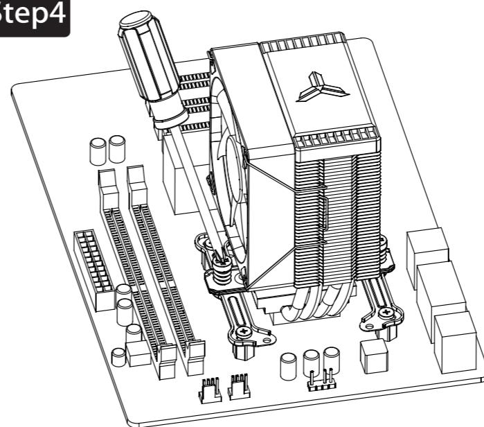
Place the cooler on the CPU while aligning the screws to the backplate mounting points, secure with screwdriver.
