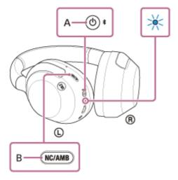
When the initializing is complete, the indicator (blue) flashes 4 times ( • - • - • -).
