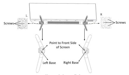
Figure 2-2 Install the Base
