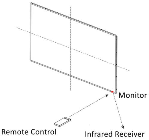
Figure 3-1 Aim at the Infrared Receiver
