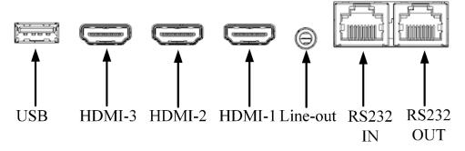
Figure 1-2 Interfaces on the Rear Panel
