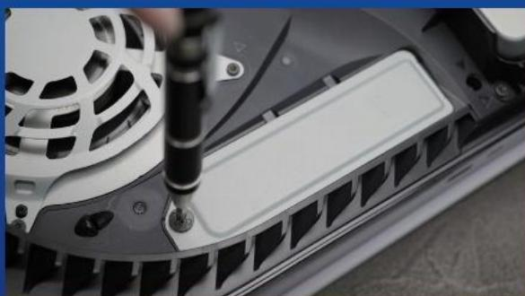
**4. LOOSEN THE SCREW TO REMOVE THE EXPANSION SLOT COVER.**
