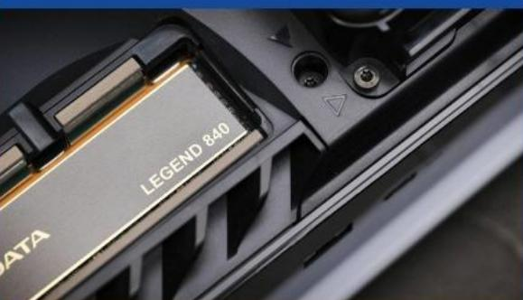
**8. CLICK THE GOLD CONNECTOR OF THE SSD INTO THE MATCHING INPUT NOTCH.**
