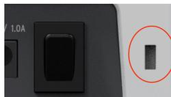
We've included a Kensington lock slot on the far right edge of the back panel so you can secure it to the surface of your choice.
