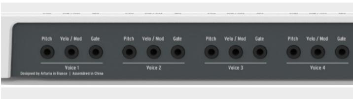
The Pitch CV output is mostly used to control the pitch of an external voltage-controlled oscillator (VCO).
