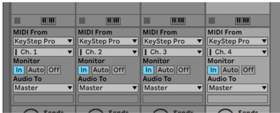
In this setup, the four KeyStep Pro tracks will play on the four corresponding Ableton tracks.
