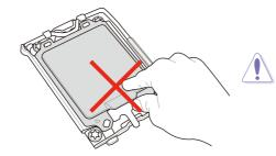
Do not remove the PnP cap yet from the CPU socket. Doing so may bend the pins of the socket.
