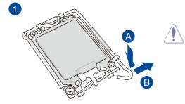
Take caution when lifting the load lever, ensure to hold onto the load lever when releasing the load lever. Letting go of the load lever immediately after releasing it may cause the load lever to spring back and cause damage to your motherboard.
