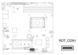
2. Align and connect the PFR module to the PFR module connector.
